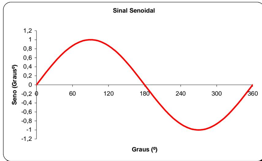
$$\text{Período} = 360^\circ, V_p = 1 \therefore v(\theta) = V_p \cdot \text{sen}(\theta) [\text{volts}] \rightarrow \boxed{1 \cdot \text{sen}(\theta) [\text{volts}]}$$
